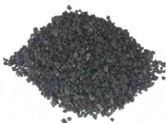
Activated carbon granules
